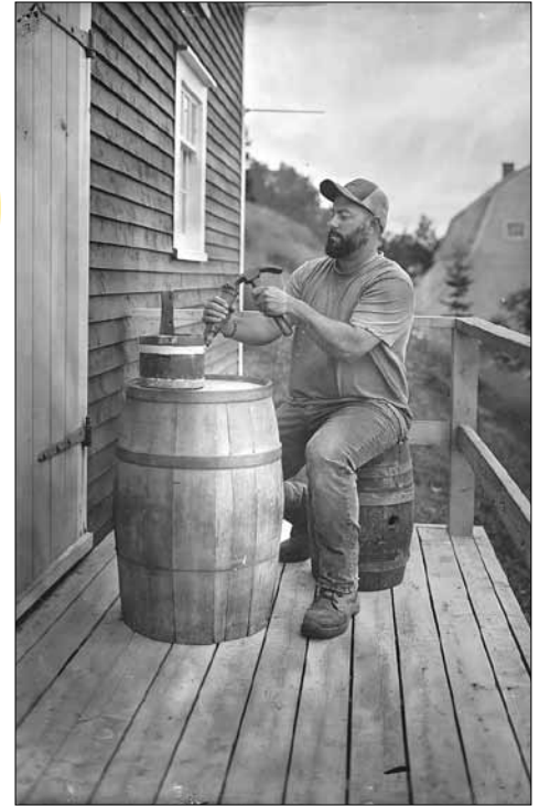
John DiMartino Jr. photo Taken while working on his occupational tintype work in Newfoundland, DiMartino photographed Darrin Hookey, a cooper at the Trinity Historical Society, where they have a working cooperage. Hookey is making a small pail used to bail water from a dory or skiff.
